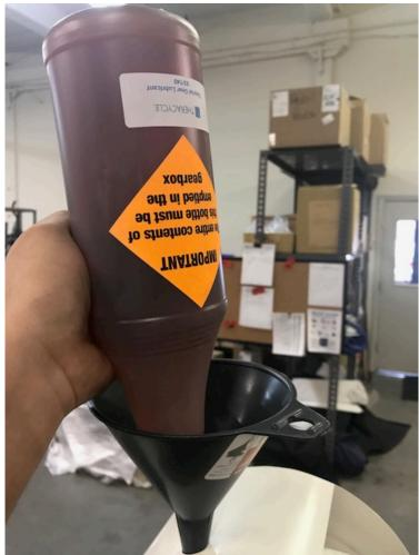
• Once the you fill the gear box with the quart of oil, use the Flat-Head Screwdriver re-install the oil fill plug to the gearbox. Lastly, re-install the plastic press fit cap to the upper bike shroud.
