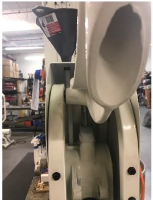
Fill the gear box with the new quart of oil. Due to the oil being very thick it will take up to 15 – 20 minutes to fill. Make sure you fill the gear box with the entire bottle of oil. You will have to fill the funnel up several times and wait as it drains into the gear box.
