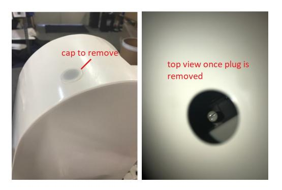
• Insert the Flat-Head Screwdriver into the hole and use it to remove the gearbox fill plug.
