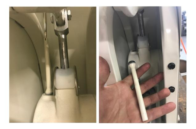
• Once the fill plug is removed, insert the funnel through the top hole of the upper shroud and into the oil fill hole.
